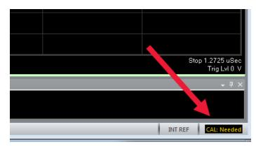
When a calibration is needed, user can either launch it from **Utilities > Calibration** or by clicking on **CAL:** Needed.
